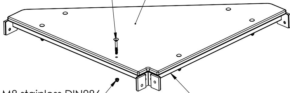
Cap lock nut M8 stainless DIN986
