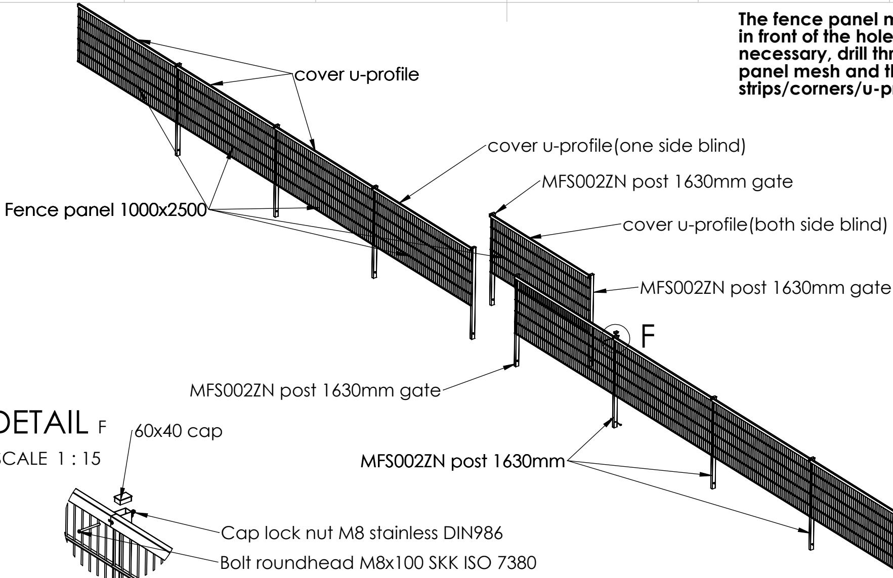
The fence panels are connected to the post with U-clamps. There are 3 U-clamps per 1m of fence!!!
