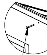
Cap lock nut M8 stainless DIN986
