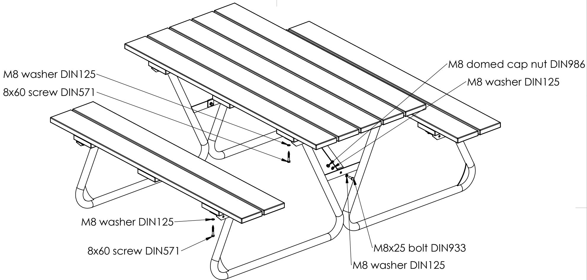
**Drill 5mm holes before attaching the screws!!**
